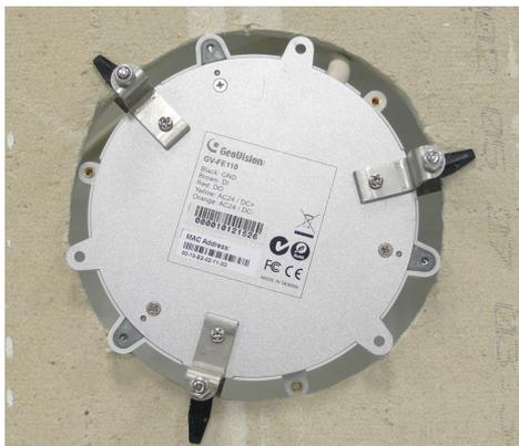
6. From the front side of the camera, tighten the screws.
