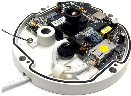
7. Connect the supplied data cable if needed.
