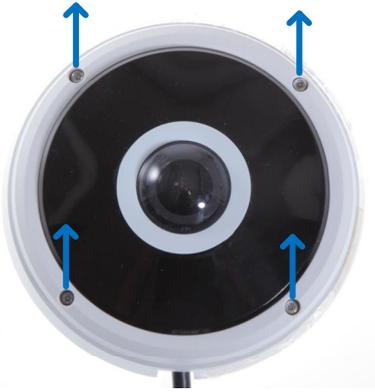
7. Secure the camera to the back plate by tightening the 4 screws as shown below. The cables can be threaded through the cable opening on the side or through the ceiling board.
